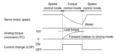
Note: When the start signal (ST1 · ST2) is switched off as soon as the mode is changed to speed control, the servo motor comes to a stop according to the deceleration time constant.
